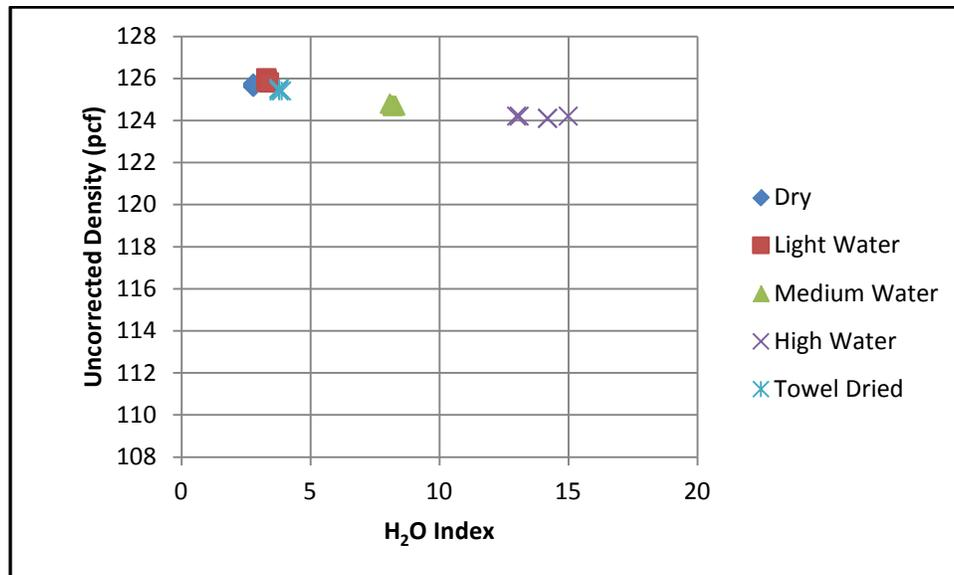
Figure 40. PQI 301 Density Change with Moisture on Slab 11
