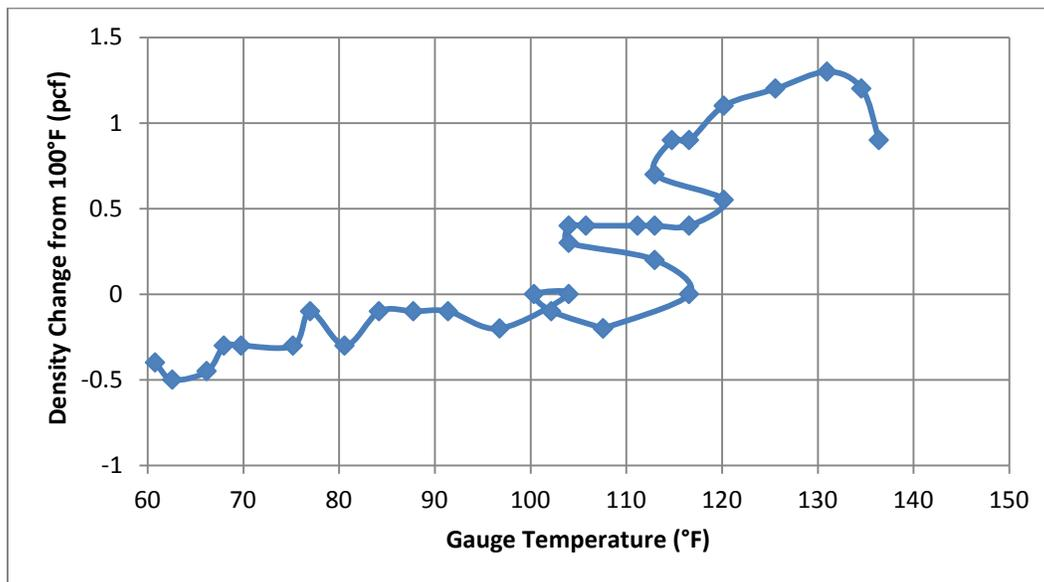
Figure 55. PQI 380 Temperature Test on Slab 10
