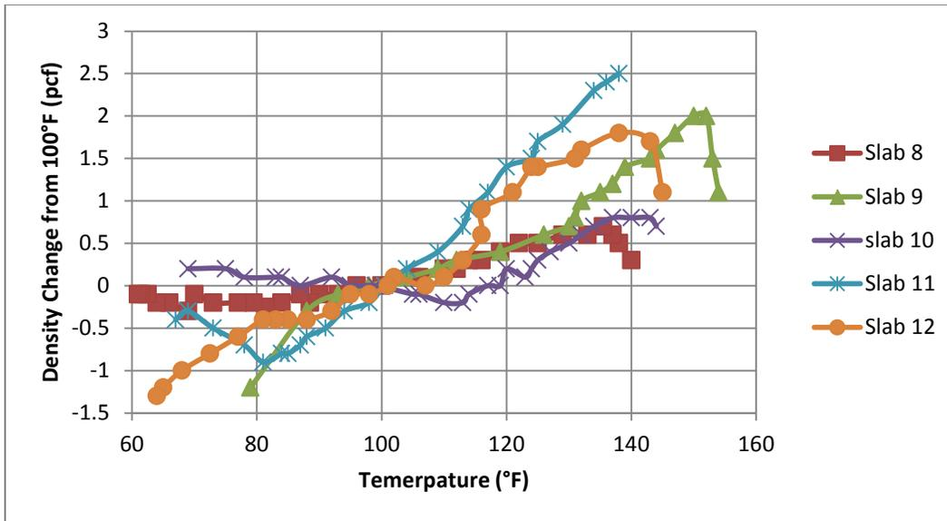
Figure 54. PT New Temperature Tests on 2013 Slabs
