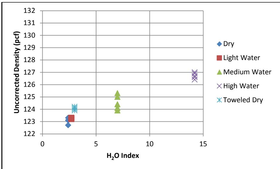
Figure 38. PQI 380 Density Change with Moisture on Slab 10
