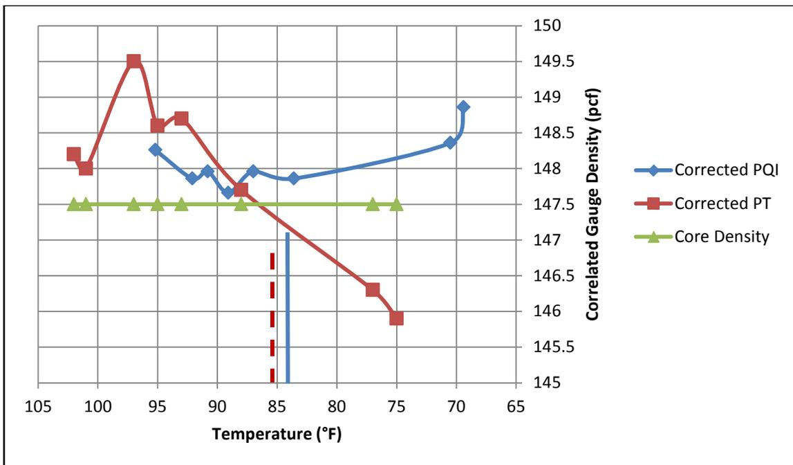
Figure 57. Field Temperature Test Results from US-12 Orofino
