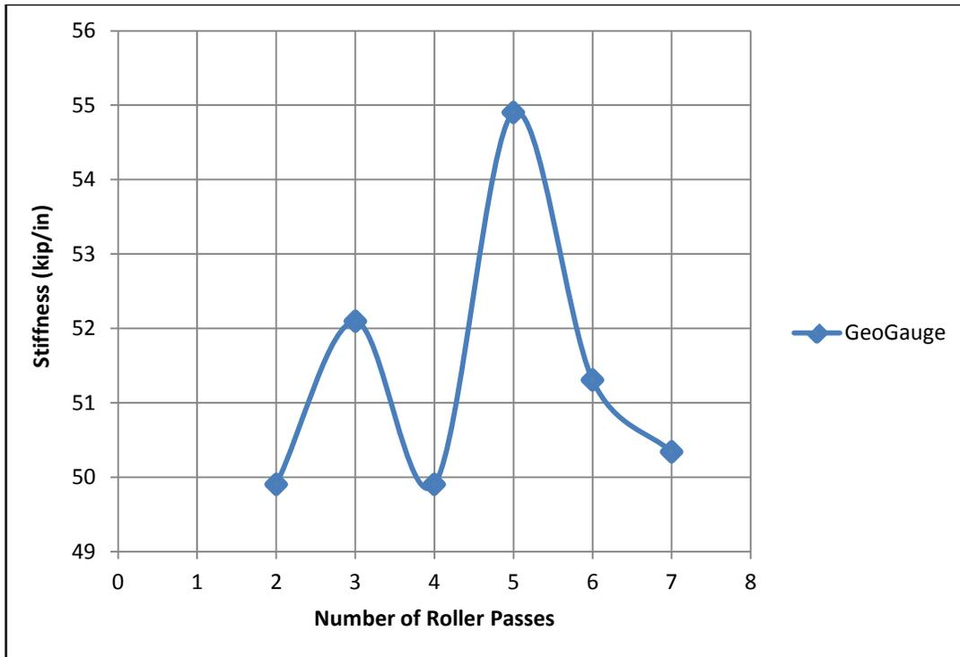
**Figure 105. GeoGauge Stiffness Values for Roller Pattern Setup at US-95 Cottonwood Site**
