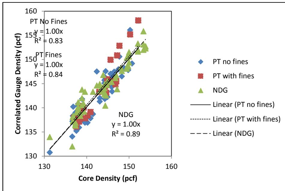
Figure 19. PT and NDG Validation with Core Densities
