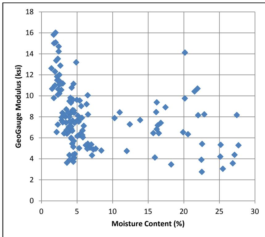
Figure 97. GeoGauge Modulus vs. Oven Moisture Content
