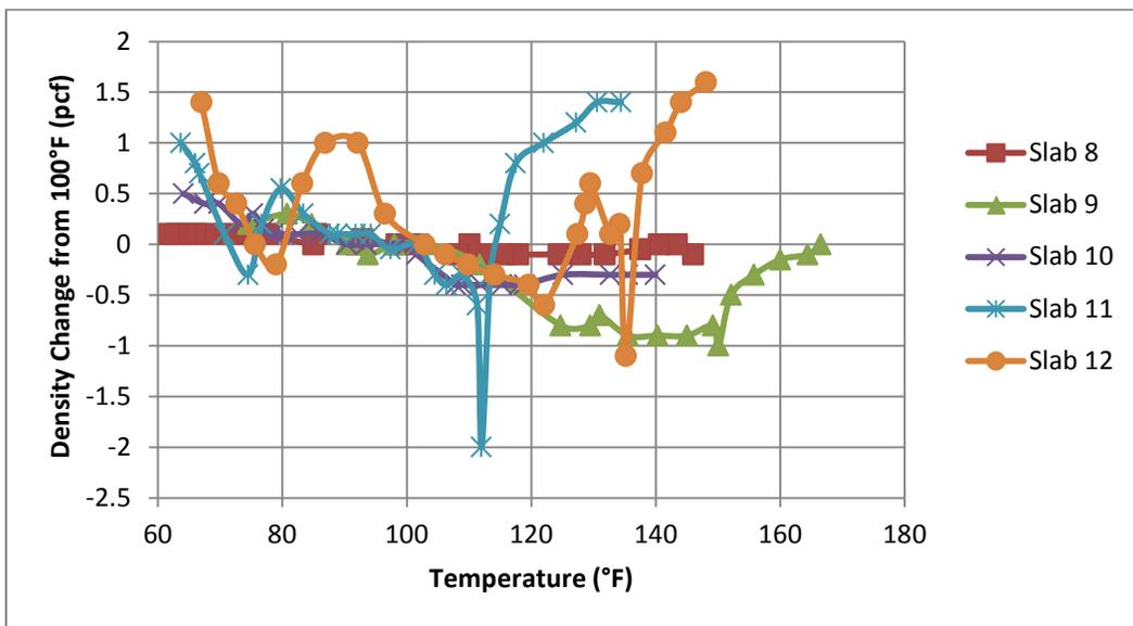
Figure 51. PQI 301 Temperature Tests on 2013 Slabs
