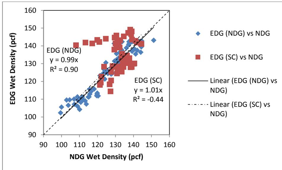
**Figure 72. Wet Density Validation: EDG vs. NDG**
