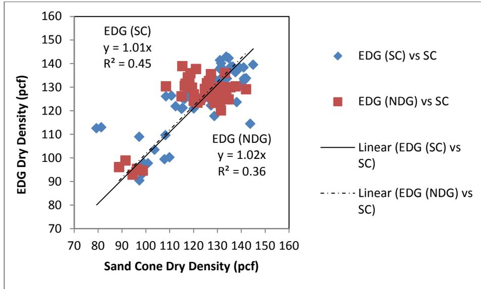
Figure 66. Dry Density Validation: EDG vs. Sand Cone
