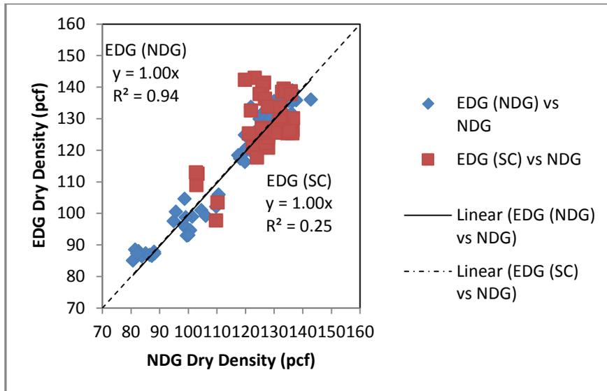
Figure 62. Dry Density Validation: EDG vs. NDG
