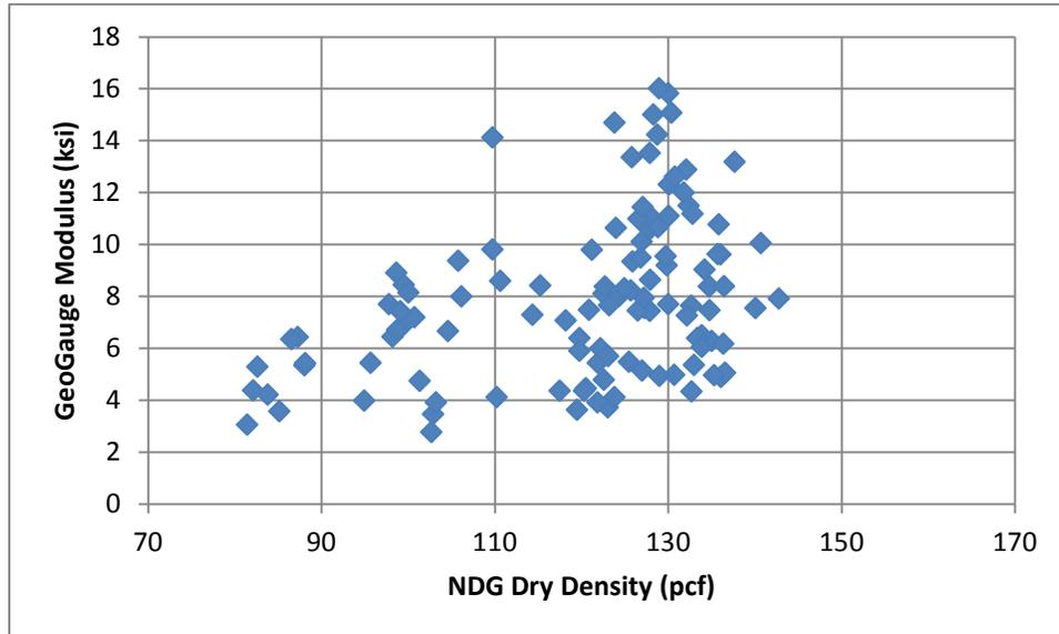
Figure 95. GeoGauge Modulus vs. NDG Dry Density
