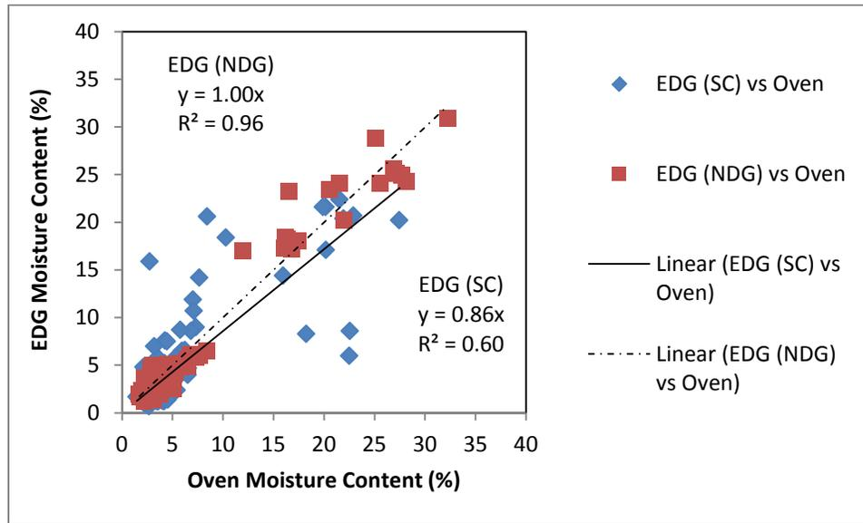
Figure 68. Moisture Content Validation: EDG vs. Oven
