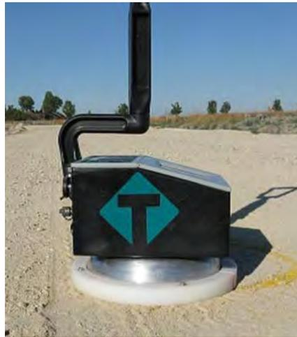
**Figure 7. Soil Density Gauge 200**
