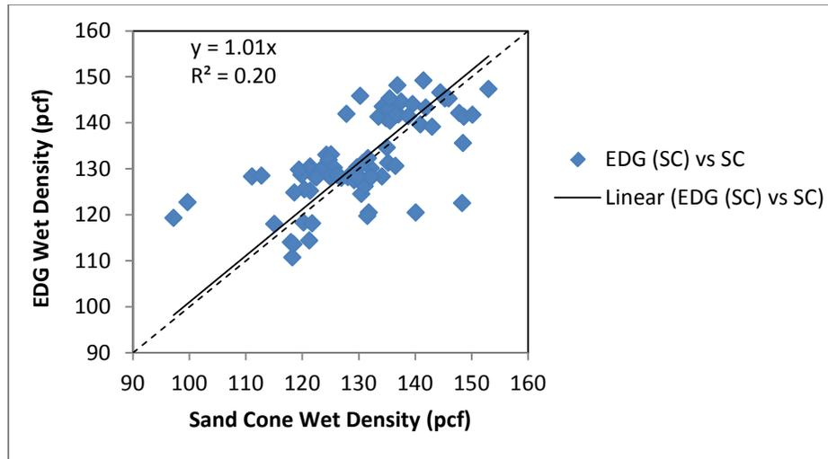
Figure 76. Wet Density Validation: EDG vs. Sand Cone
