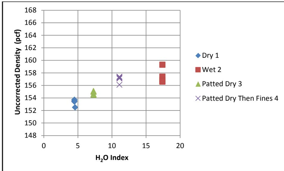
Figure 34. PQI 380 Density Change with Moisture on Slab 9
