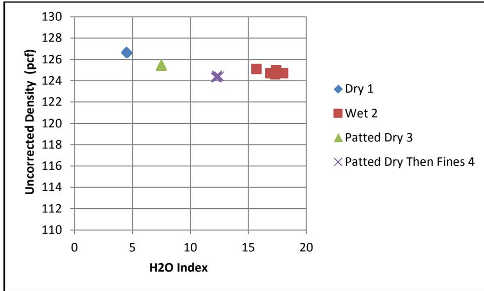
Figure 32. PQI 301 Density Change with Moisture on Slab 9
