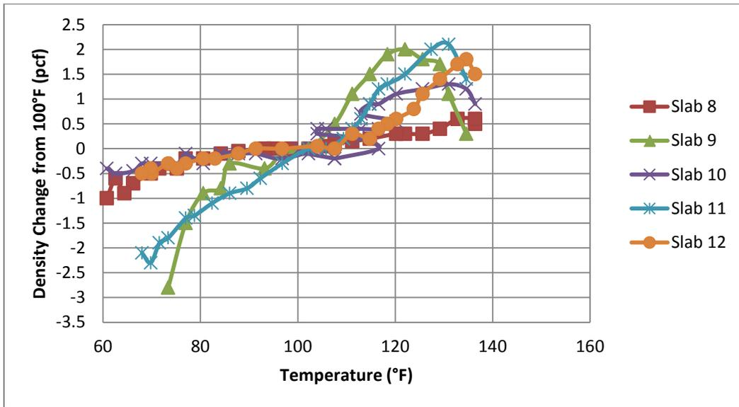
Figure 53. PQI 380 Temperature Tests on 2013 Slabs
