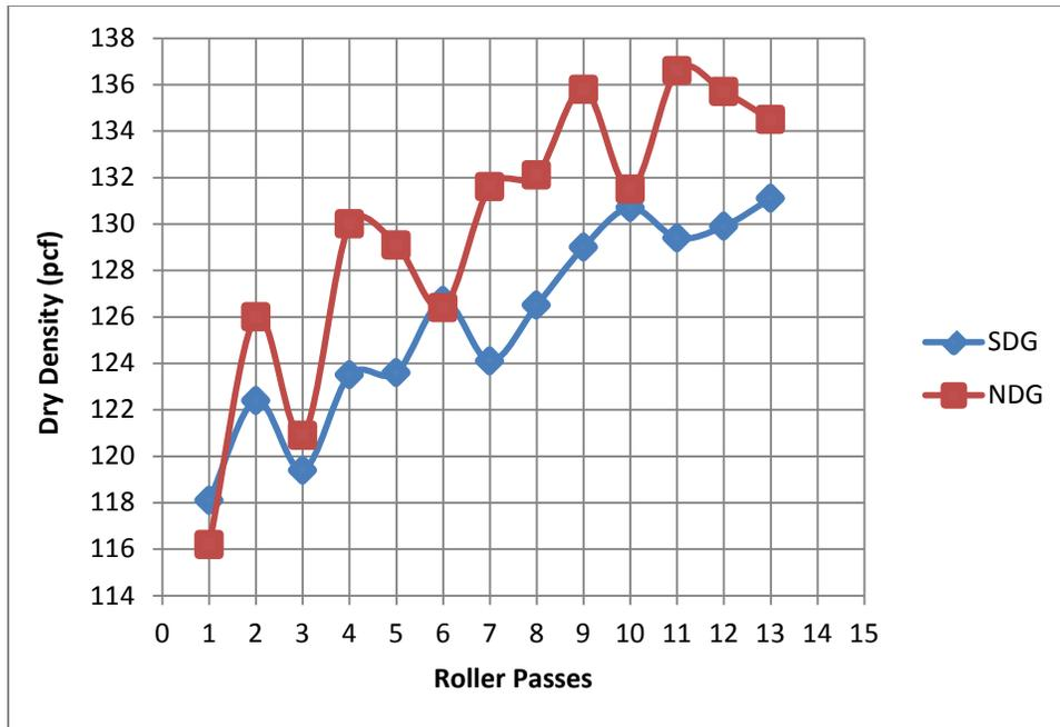
Figure 100. Comparison of NDG and SDG Density Values for Roller Pattern Setup 3 at US-95 Wilder Site
