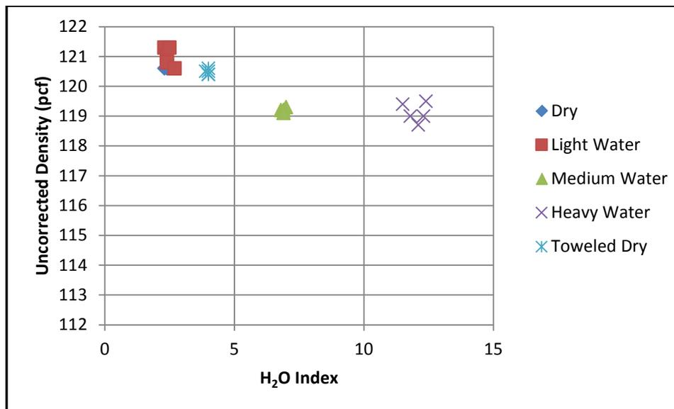
Figure 36. PQI 301 Density Change with Moisture on Slab 10
