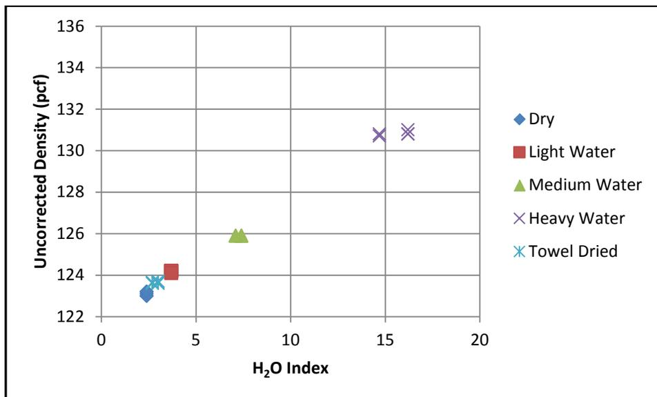
Figure 46. PQI 380 Density Change with Moisture on Slab 12
