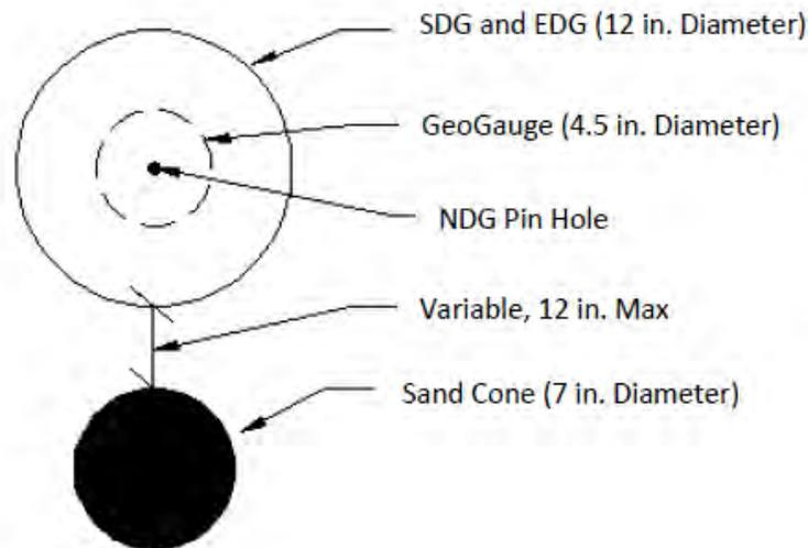
**Figure 16. Unbound Field Testing Pattern**
