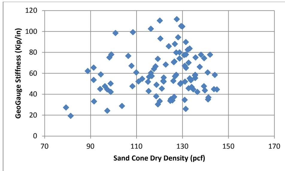
Figure 93. GeoGauge Stiffness vs. Sand Cone Dry Density
