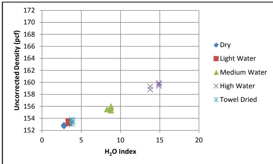
Figure 42. PQI 380 Density Change with Moisture on Slab 11
