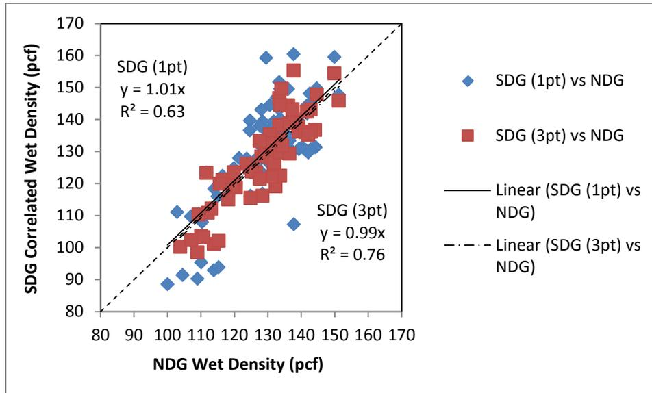
**Figure 73. Wet Density Validation: SDG vs. NDG**
