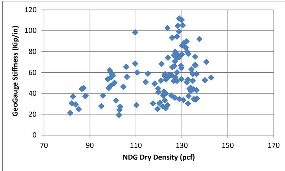
Figure 92. GeoGauge Stiffness vs. NDG Dry Density
