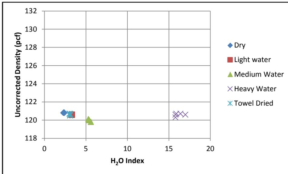
Figure 44. PQI 301 Density Change with Moisture on Slab 12
