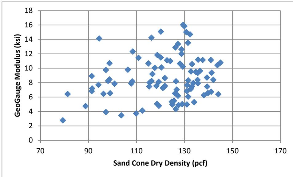
Figure 96. GeoGauge Modulus vs. Sand Cone Dry Density
