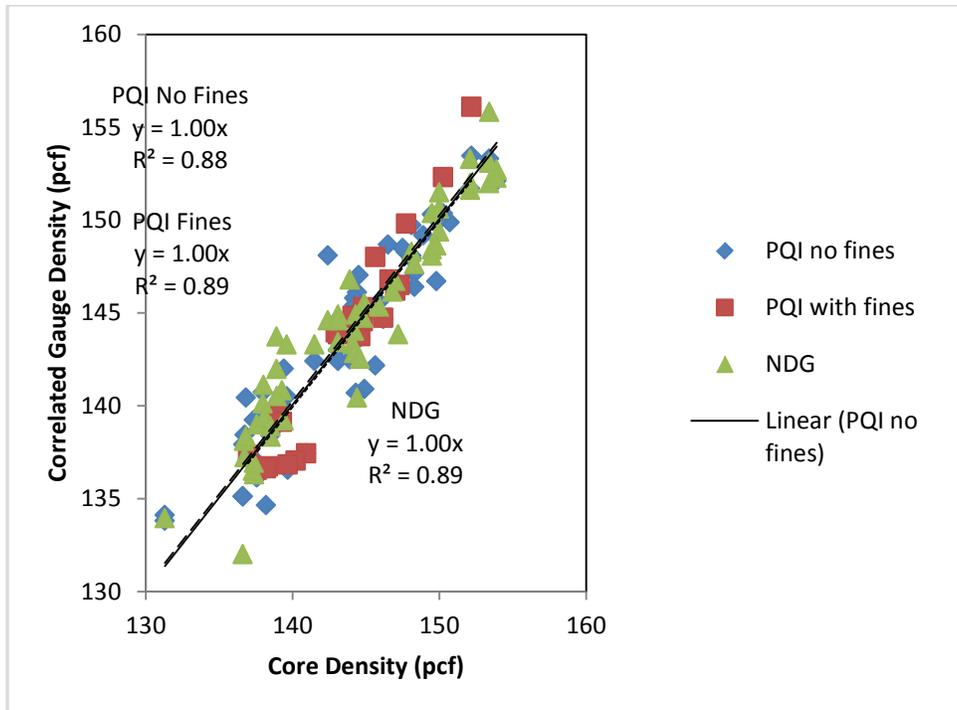
Figure 18. PQI and NDG Validations with Core Densities
