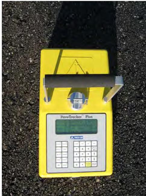
Figure 5. Troxler PaveTracker™ Model 2701-B
