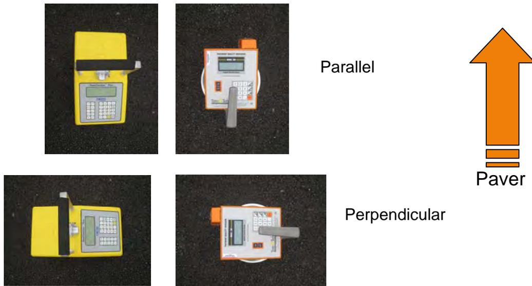
Figure 10. Parallel and Perpendicular Gauge Orientation
