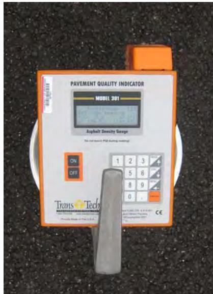
Figure 4. Pavement Quality Indicator™ (PQI) Model 301
