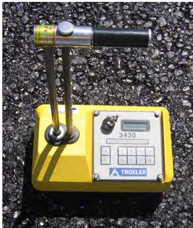
Figure 2. Troxler Model 3430 Nuclear Gauge
