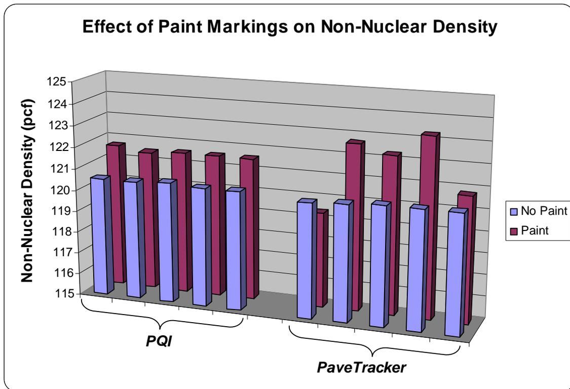
Figure 24. Effect of Paint Markings on Non-Nuclear Density
