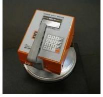
strict licensing and usage procedures, take several minutes to get data, and have limitations in their accuracy. Further, the time required by nuclear devices to obtain useful density data limits their in-process, Quality Control (QC) effectiveness during pavement construction.
